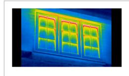
Thermal differential visible at the junction between the panes and the window frames; these junctions and their seals are often the areas of windows which deteriorate first, resulting in warping of the window frames, energy inefficiency, draughts, and condensation related problems (mould and water damage staining).
