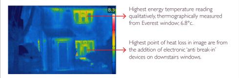
Whilst the windows are still the least energy efficient part of the building because, by their very nature window frames thermally bridge the internal and external environment, the new Everest window system provide a significant improvement in thermal efficiency, and will help reduce the propensity for condensation as well as facilitate in the reduction of energy bills.
